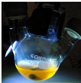
Figure 6: Three-neck flask with ZnTe/ZnSe QDs with two shell monolayers shortly after the reaction under UV light.
