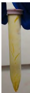
Figure 8: Washed ZnTe/ZnSe QDs in centrifuge tube after washing before being dispersed in hexanes.
