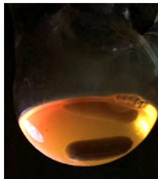
Figure 11: Three-neck flask with ZnTe/ZnS QDs with three shell monolayers under UV light shortly after the reaction.
