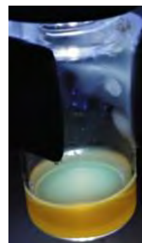
Figure 9: ZnTe/ZnSe QDs in a scintillation vial with three shell monolayers dispersed in hexanes under UV light.
