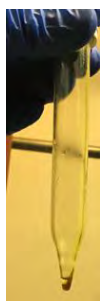
Figure 12: Washed ZnTe/ZnS QDs in centrifuge tube after washing before being dispersed in hexanes.
