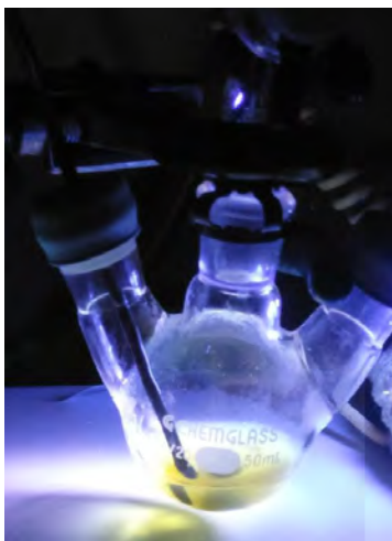
Figure 5: Three-neck flask with ZnTe-nanoparticle cores under UV light shortly after reaction.
