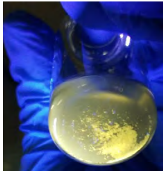
Figure 3: Oxidized ZnTe-nanoparticle cores dispersed in hexanes a week after synthesis under UV Light.
