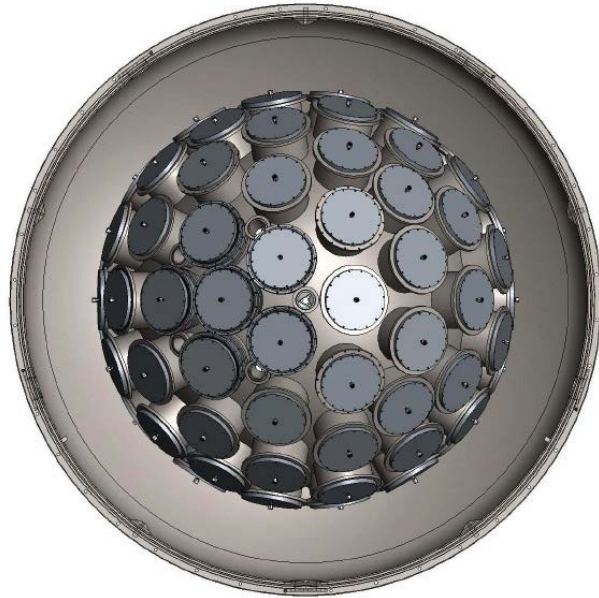
Figure 7: A cut away view of the MiniCLEAN detector's inner vessel and the surrounding outer vessel. The top hats of the 92 optical cassettes along with the calibration ports are visible.
