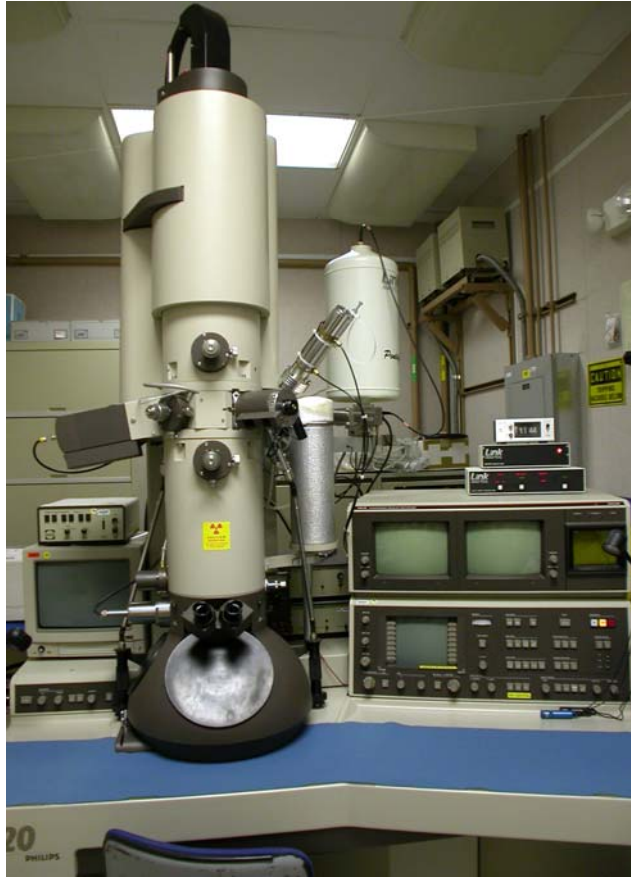
Figure 4: Our 200 keV Philips CM20 Transmission Electron Microscope.
