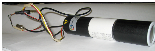
Figure 16. The newest version of the PMT has no high-voltage base.
